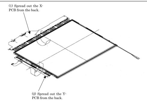
Figure 4-54 Replacing TMD fluorescent lamp (WXGA) (4)
